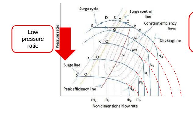
No capping of the speed lines with the speed of sound, because the speed of sound of hydrogen is about three times that of natural gas.
